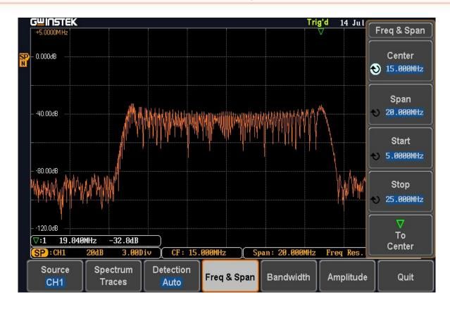
The user is allow to set Start Frequency, Stop Frequency, Center Frequency, and Span to intuitively and rapidly identify the desired frequency range
