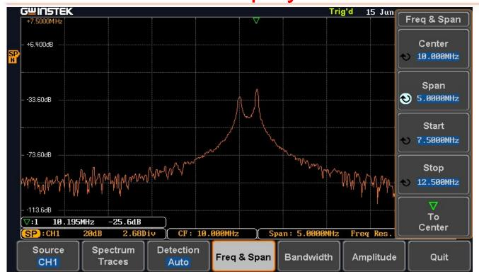
The input signal is FSK  $500 \text{mV}_{pp}$  sine wave
