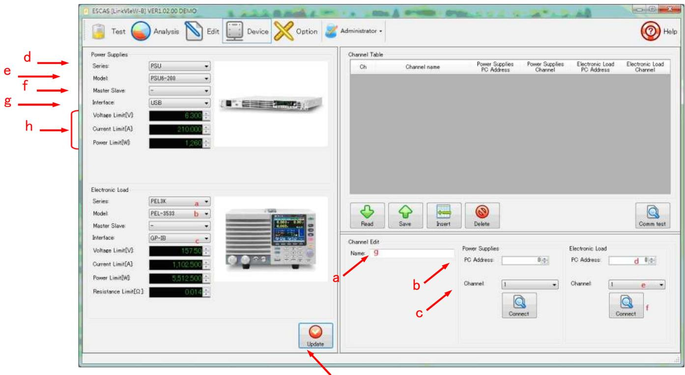
Set up PC address of equipment which will be examined and a channel of Power Supply or Electronic Load.
