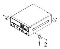
4. Attach the front plate and handles to the bottom cover using the 594B-W4010NS1 screws.
