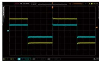
Linear CC mode, PWM 10A 2.5Hz
