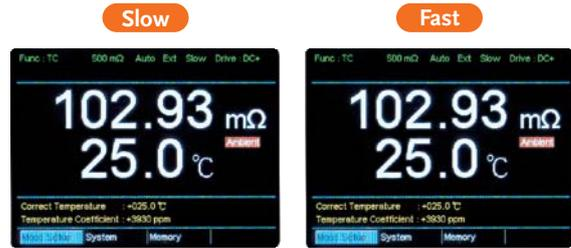
GOM-804/805 has two measurement speed selections, which are Fast reaching 60 readings per second, and Slow 10 readings per second. A major departure from the past, users, in the past, had to juggle between speed and display resolution. GOM-804/805 will not affect resolution despite of any speed selections and will maintain the highest display digits. In other words, reading resolution will not be changed by changing speed and the display digits remain the same.
