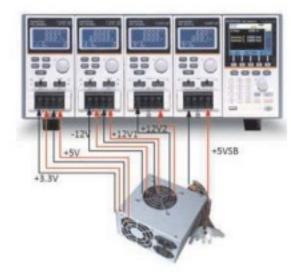
Test Diagram for ATX Power Supply
