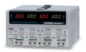
The GPS Series linear power supplies have 2-4 independent output channels, 180W to 200W output, overload and reverse polarity protection as well as an output ON/OFF switch for safety. The tracking mode switches allow voltage/current to be output in parallel or series and the intelligent fan reduces noise. The GPS-Series is an entry level general purpose power supply recognized for their affordability in education, laboratories and industry.
