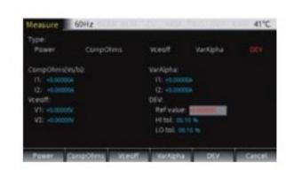
GSM-20H10 provides five built-in calculation functions: Power, Offset Compensation Ohms, Voltage Coefficient, Varistor Alpha, and Percent Deviation.
