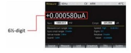
GSM-20H10 provides a measurement accuracy of up to 0.012%, and provides a meter display function of up to 6½ digits, allowing users to have more accurate results when measuring small signals...
