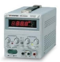
The GPS-Series is a single output, 54W to 90W, linear DC power supply. The GPS-Series has digital display meters with varying power outputs. The GPS-Series features overload and reverse polarity protection as well as high regulation and low ripple/noise that are maintained at 0.01% and < 1mVrms, respectively. Continuous or dynamic internal load selection accommodates applications such as pulsed current. Remote control terminals offer programming and operation from an external device.
