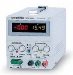
The SPS-Series is a single output, 360W, switching DC power supply. OVP protects the SPS-Series and their loads from unexpected conditions. High regulation is maintained at 0.01%. Remote sensing adds an extra level of precision by compensating cable losses between loads. Turning the output On/Off from external device is available through Remote control terminals. The GPS-Series is an ideal solution for power-efficient bench-top or portable applications requiring high regulation.
