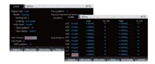
GSM-20H10 has three built-in Pass/Fail limit line tests with a total of 11 sets.
