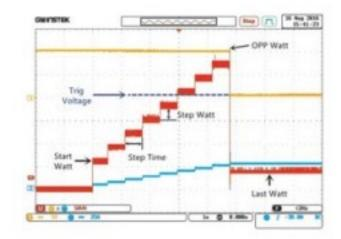
OPP test Automation for DUT (Power Supply), Provide users with high resolution OPP measurement values to verify DUT's OPP activation point. Provide users with measurement results so as to help them determine whether DUT's actual OPP activation point meets the regulations. Test the value of OPP by setting power increment from start power to stop power. OPP's activation point can be accurately measured.
