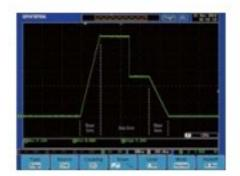
Ramp function of PEL-3000E Series is able to set the current transition. When turned on, the current takes on a slope form; when turned off, the current takes on a step form.
