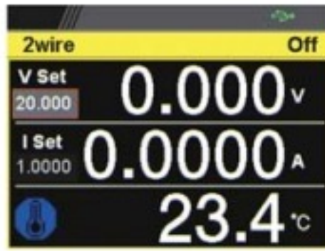
Blue: Temperature Control on with no GTL-205A Connected
