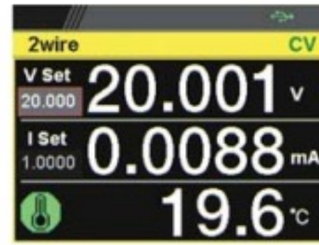
Green: Output Safe is Activated and Output is on with GTL-205A Connected
