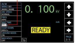
Wait Time Indicator While the WAIT TIME is set, the indicator of WAIT TIME will be shown on the display in the set duration during a test progress for clear identification for user.
