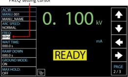
3. Use the scroll wheel to set the test frequency.
