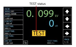
3. The test will start by showing the ongoing ramp up time followed by the ongoing test time and the ongoing ramp down time. The test will continue until the test is finished or stopped.
