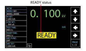
2. Press the START button when the tester is in the READY status. The manual test starts accordingly and the tester goes into the TEST status.
