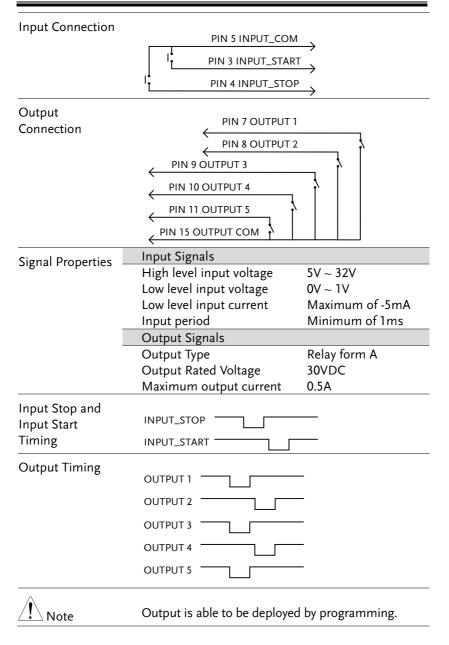
Using the SIGNAL I/O to Start/Stop Tests
