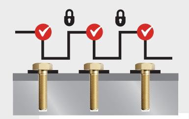
Restart Delay in OK/NOK Cycles: The Restart Delay function (also known as Rehit Prevention Mode) locks the tool, which disables the trigger for a specified period of time, and prevents operation when running an OK or NOK Tightening Cycle.
