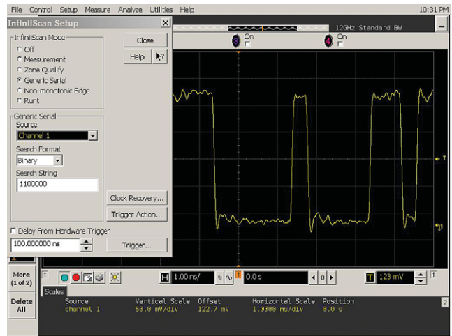
Figure 7. InfiniiScan’s generic serial finder is used to isolate a specific portion of a high-speed serial data stream.
