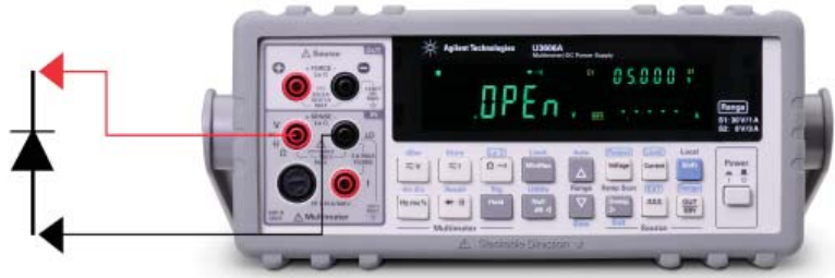
Figure 2. Reverse-biased condition in a diode
