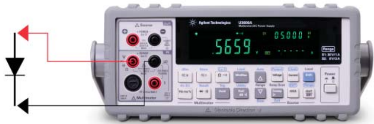
Figure 1. Forward-biased condition in a diode
