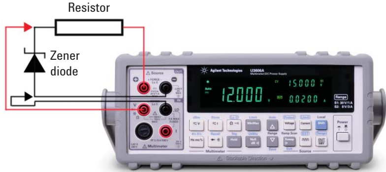
Figure 5. Zener diode test using the U3606A
