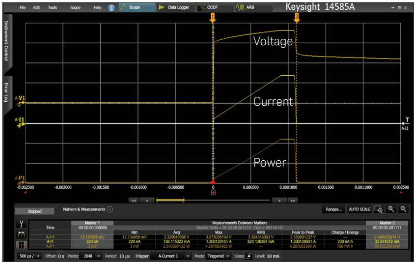
Figure 9-1. HBLED fast ramped current forward voltage test
