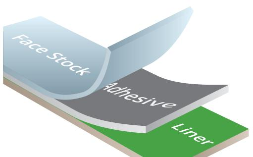
**Face Stock:** 2.4 mil topcoated gloss white polyimide film offering excellent chemical resistance combined with superior high heat resistance. The material will not curl and is designed to survive high temperatures of lead-free solder processes.
