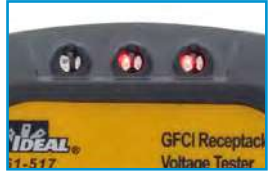
Red Lights Indicate Incorrect Wiring
