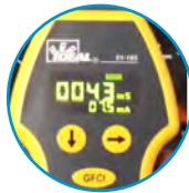
Trips GFCI at 6mA or 30mA
