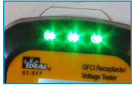
Green Lights Indicate Correct Wiring
