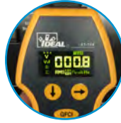
Displays neutral to ground voltage
