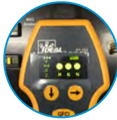
Displays H N G polarity
