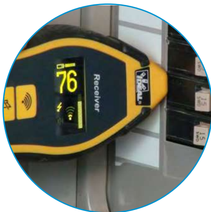
Finding Breakers or Fuses
