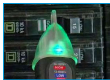
Power On Indicated by a Green LED
