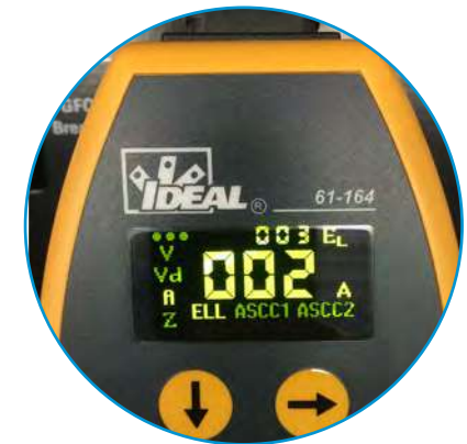
Estimated Load on Line in Amps
