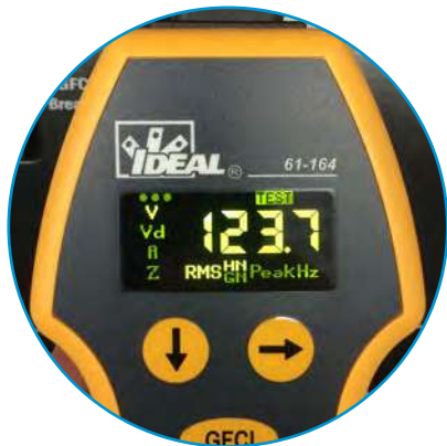
True RMS Line Voltage
