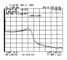
Sinewave, squarewave, and PRBS modulation each cause different chirp levels. But, large amounts of amplitude modulation from any source will cause large FM deviations.
