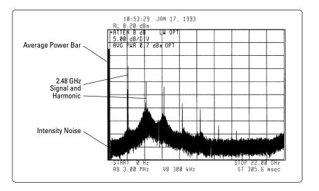
to rely on data-sheet RIN specifications to predict the effects of laser noise within an operating system.
