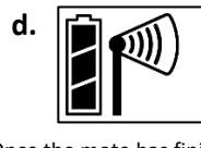
Once the mote has finished joining the network, the "x" icon is removed and the channel count on the station LCD increases by four (three for soil moisture, EC, and temperature, and one for the mote battery).
