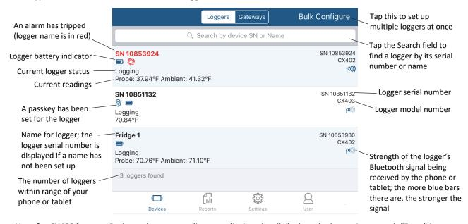
**Note for CX400 loggers:** Probe and sensor readings are displayed as "--" when the logger is stopped. "Error" is displayed if the probe is disconnected from the logger. Probe and sensor readings are updated at a different rate than the logging interval and may not match what is currently displayed on the logger LCD.
