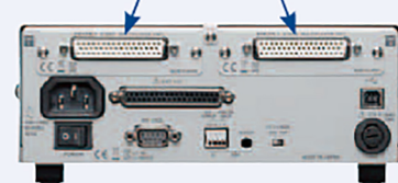
Pictured: Back of the RM3545-02 with two Z3003 units (optional feature) installed
