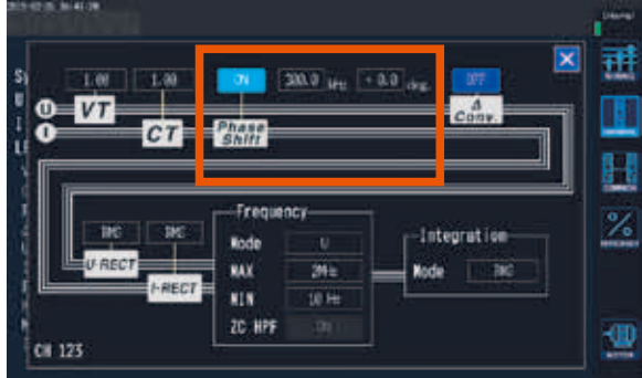
Enter phase calibration values for each frequency to correct high-frequency phase characteristics.
