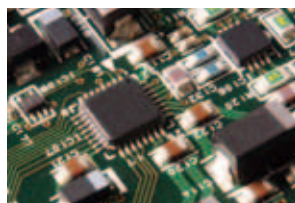
Input amp with integrated A/D converter
