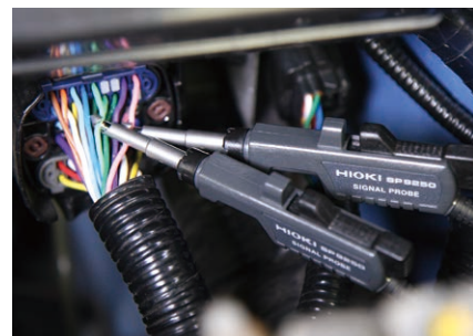
Undamaged wires for easy and safe measurement
