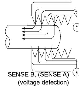
Fig. 4. Measurement with L2101 Clip Type Lead
