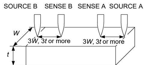
Fig. 7. Probe positions on wider/thicker measurement target
