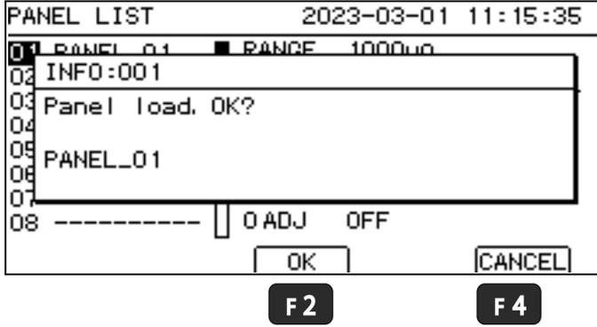
**F2** Load the panel and switch to the Measurement screen (you can also do this with the **ENTER** key).
