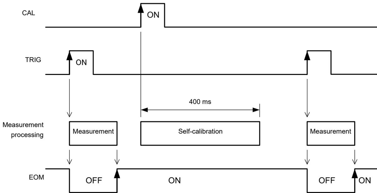
**If the TRIG signal is received during self-calibration**
