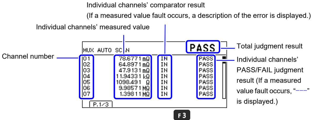
Scan measurement can be stopped by pressing **F3** [STOP] during scanning.
