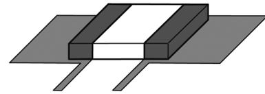
Fig. 10. Current sensing resistor mounted on a printed circuit board
