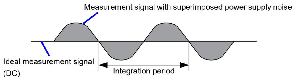
Fig. 4. Noise caused by a commercial power supply
