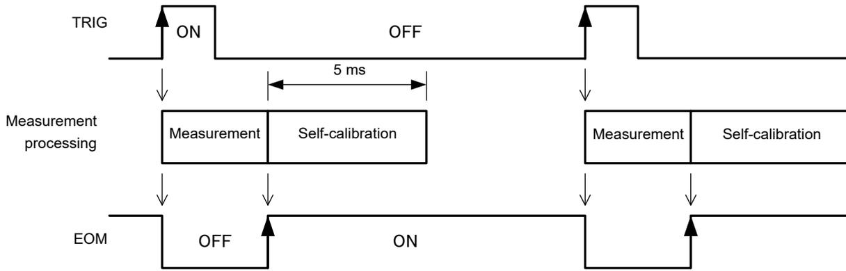
**If the TRIG signal is received during self-calibration**
