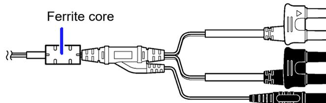
Fig. 3-1. Noise countermeasures at the measurement lead
