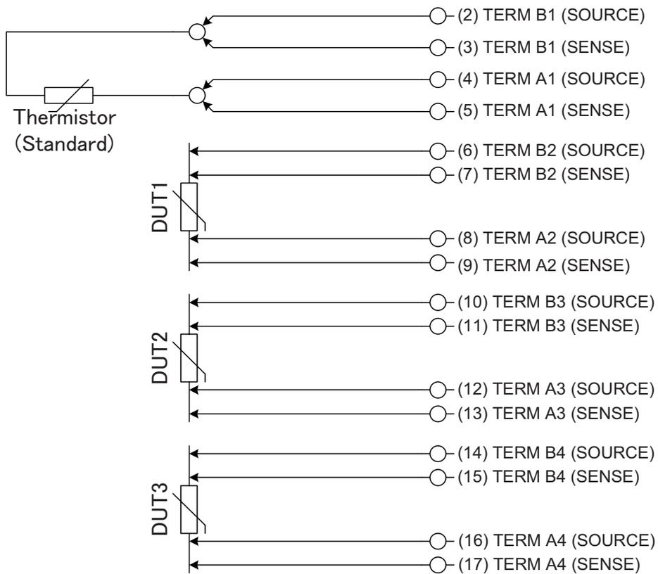
**Using channel 1 (thermistor) measurement results as the comparator reference value**
