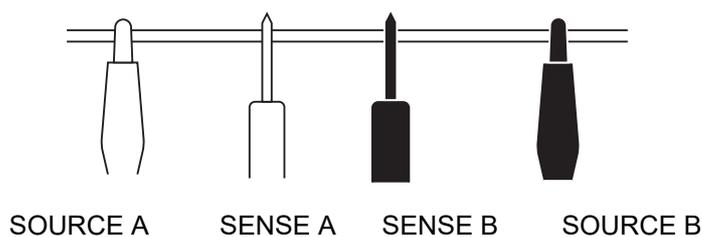
The SENSE terminals are placed to the inside of the SOURCE terminals.
