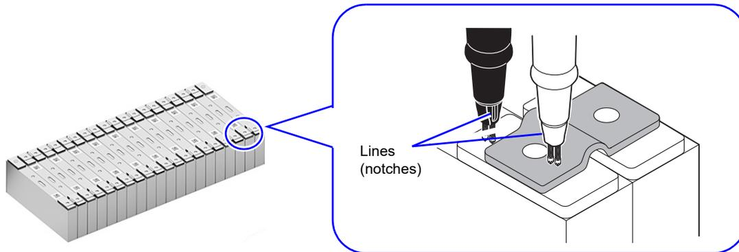
Connect the leads so that the lines (notches) on their bases face inward to each other.
