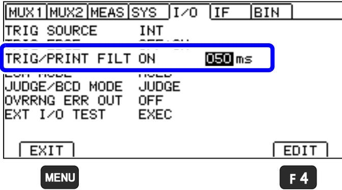
**1** Move the cursor to the setting you wish to configure. Make the value editable with the **F4** key.
