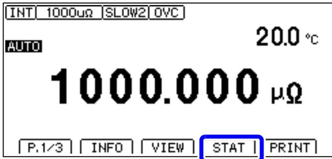
When statistical calculation is ON, **F3 [STAT]** will be displayed when the **MENU [P.1/3]** display is active.
