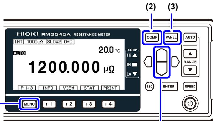
When the measurement terminal setting is MUX (multiplexer): Select the channel.
