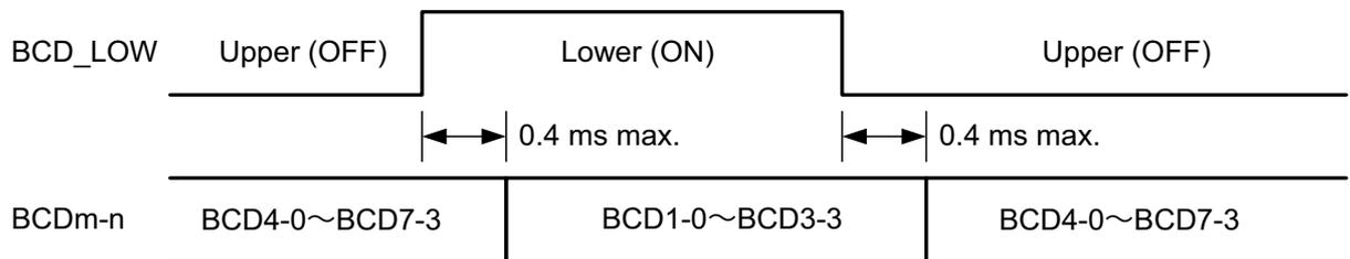
If the response of the input circuit in the controller is slow, inserting more than 0.4 ms of wait processing may be required after the BCD\_LOW signal is controlled.
