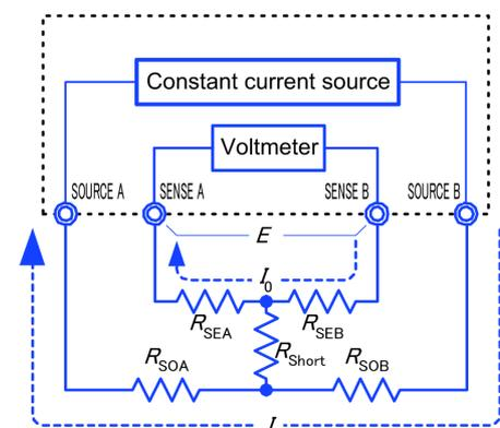
$$\begin{aligned} E &= (I_0 \times R_{SEB}) + (I_0 \times R_{SEA}) \\ &= (0 \times R_{SEB}) + (0 \times R_{SEA}) \\ &= 0 \text{ (V)} \end{aligned}$$
