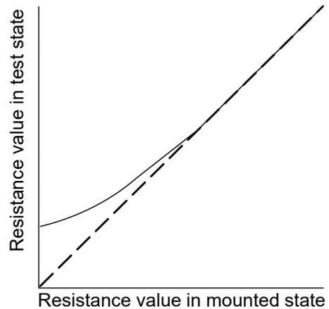
Fig. 14. Difference between mounted state and test state
