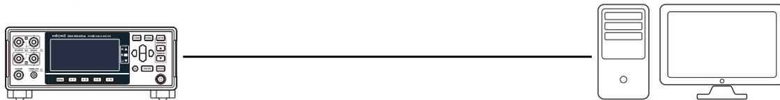
The instrument can be controlled with communications commands by creating a program with a TCP connection to the communications command port.
