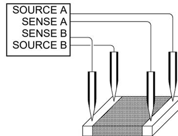
Fig. 2. Four-terminal measurement
