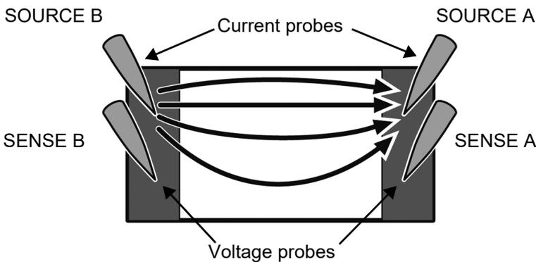
Fig. 13. Flow of current in the test state
