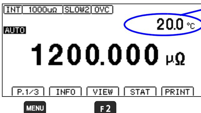
You can switch this part of the display to show nothing, the temperature, or the pre-calculation measured value.
