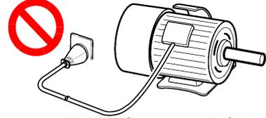
The measurement target is connected to a power supply.
