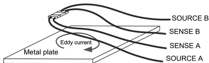
Fig. 8. Generation of an eddy current
