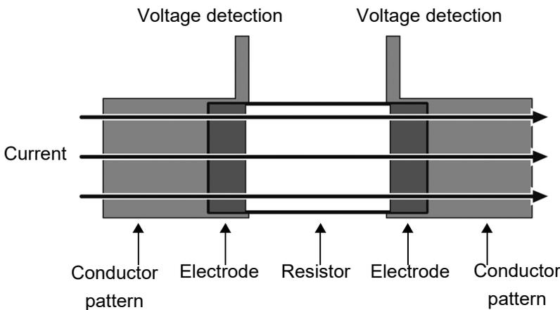
Fig. 11. Current flow in the mounted state
