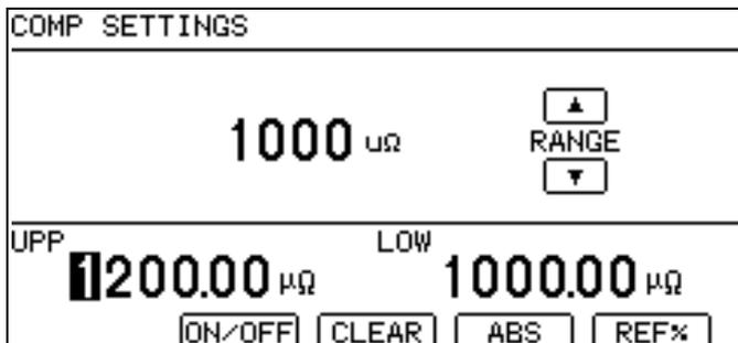
**F1** Switch the comparator function ON or OFF.
