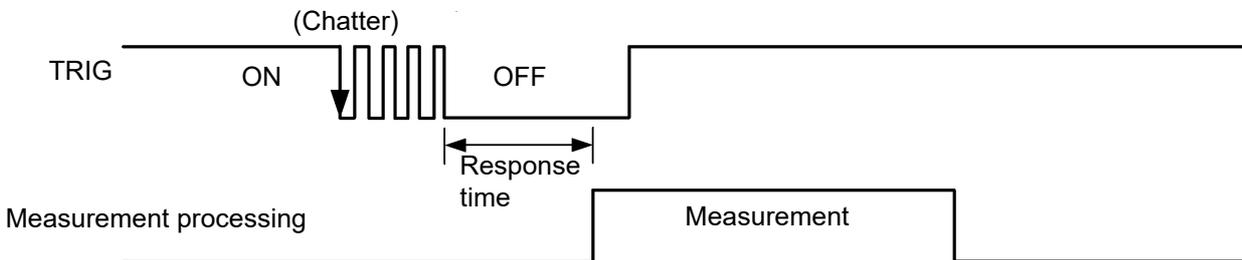
Hold the input signal until the response time elapses.
