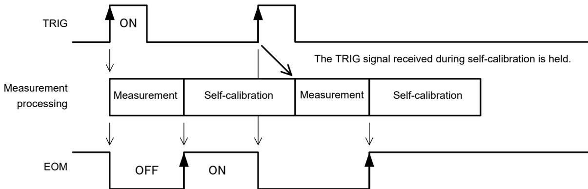
Additionally, self-calibration is performed once every second during TRIG standby operation. In the event the TRIG signal is received during self-calibration, the self-calibration is canceled, and measurement will start after 0.5 ms.
