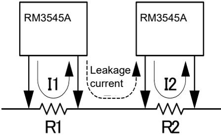
As shown in the figure below, the measurement currents from the two instruments will flow in common relative to the 10 mΩ resistance, resulting in an error.
