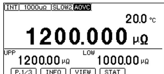
Comparator judgments are indicated only when the comparator function is enabled.
