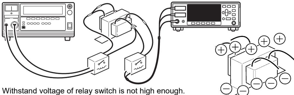
Withstand voltage of relay switch is not high enough.
