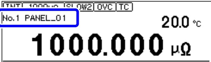
The name of the loaded panel will be displayed on the Measurement screen.
