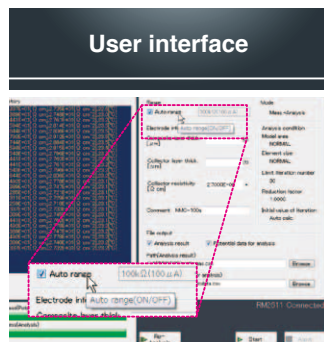
User interface Move the cursor to a parameter to view guidance including a description and valid setting range.
