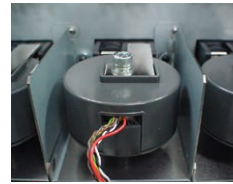
DCCT current sensor (in the PW3337)
