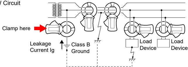
2. If leakage is occurring, investigate by lumped measurements (clamping all lines together) starting from the supply side toward the load.
