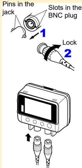
**1** Align the slots in the BNC plug on the sensor cable with the pins in the jack on the logger.
