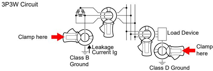
**Lumped Measurements** Clamp around all conductors together.
