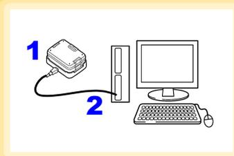
**1** Plug the USB cable into the USB port on the LR5091 (or LR5092-20), and into a USB port on the computer.
