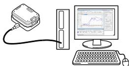
**17** Import recorded data from the logger to a connected computer. For analysis, display the data in a graph.**See:** "4.5" (p.55)
