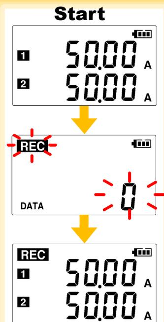
**Start** From the Measurement display, hold the **REC/STOP** button for two seconds.
