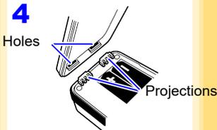
**NOTE** Note that the battery cover is designed to seal tightly to preserve dust- and drip-resistance.
