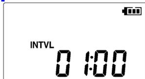
4 Select the recording interval for the logger (in this case, 1 minute).
