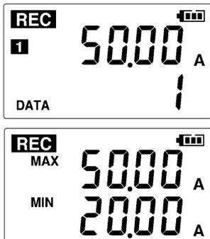
**14** Press **(+)** and **(-)** on the logger to confirm that the recording count is incrementing, and that recording data (maximum and minimum values) are displayed.
