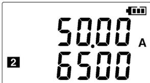
**2** Press the **(+)** and **(-)** buttons to select the clamp sensor model and measurement range.
