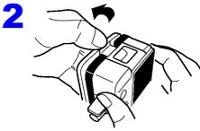
**1** Press the PUSH tab as shown, and pull the battery cover back.
