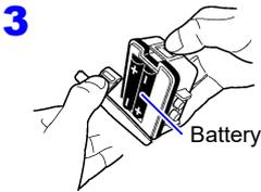
**3** Install the battery as shown.
