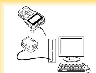
**1** Plug the USB cable into the USB port on the LR5091 (or LR5092-20), and into a USB port on the computer.
