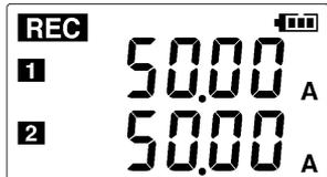
**13** Hold **REC/STOP** on the logger for two seconds to start recording.**See:** "4.3" (p.53)**14**
