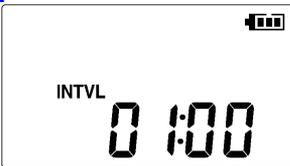
**4** Select the recording interval for the logger (in this case, 1 minutes).**See:** "Recording Interval Setting" (p.31)
