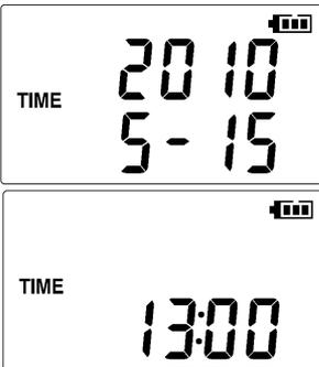
**5** Set the logger to the correct date and time (in this case, 15 May 2010, 13:00).**See:** "Real-Time Clock Setting" (p.32)
