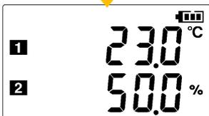
**Start** From the Measurement display, hold the **REC/STOP** button for two seconds.
