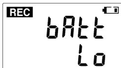
Recording is not performed while [bAtt Lo] is displayed. (Data for this period will be missing when the data is imported to a computer.) However, if you insert a new battery within approximately 30 seconds, recording will be resumed after the logger has waited for temperature/humidity sensor output to stabilize (approximately 30 seconds).
