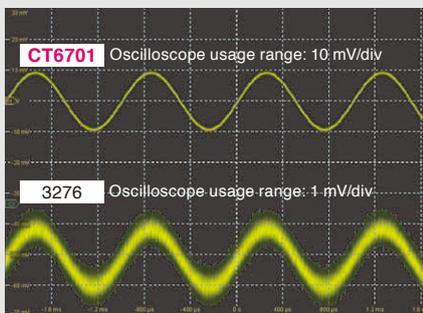
Input: 20 mA p-p, 1 kHz, sine wave
