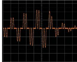
Forming machine load current
