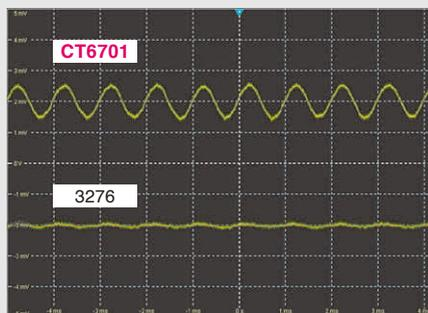
Input: 1 mA p-p, 1 kHz, sine wave
