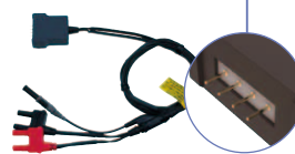
4-point probes (5.0 mm pitch)
