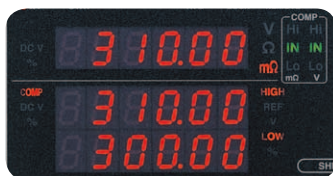
Resistance comparator settings
