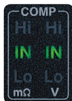
Resistance comparator settings
