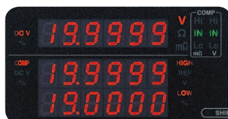
Voltage comparator settings
