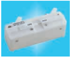
9677 SMD TEST FIXTURE Operating Frequency : DC to 120 MHz Measurable Object Size : 3.5 ±0.5 mm Dimensions : Approx. 103W × 37.1H × 47.6D mm Mass : Approx. 135 g
