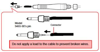
Replace the 9465-90 pin tip by inserting a new pin into the socket and pressing against a hard board or other surface to fix the pin firmly in place.
