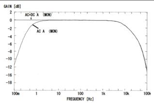
Fig. 1 Frequency Characteristics of Current Output
