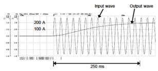
Fig. 2 Waveform of Output Response (Rise)
