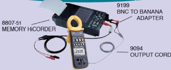
Using the external output functions of the 3284 or 3285 in combination with a HIOKI MEMORY HiCORDER enables recording of current and frequency fluctuations and recording and harmonic analysis of instantaneous waveforms. The monitor output (MON) spans a wide frequency range from DC to 20 kHz (15 kHz in the case of 3285), which allows the units to be used for electric current analysis in various fields ranging from batteries to inverters.
