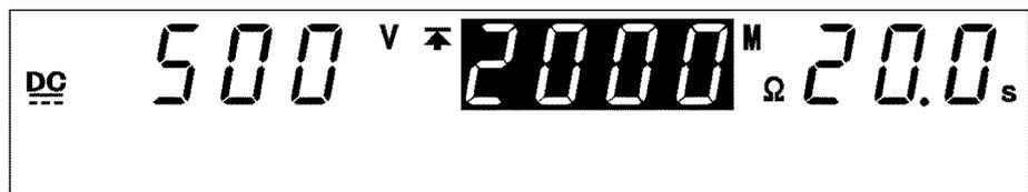
The upper-limit value is set at **2000 MΩ**. Turn it **OFF**, as it is not needed. To change to **OFF**, press the **ON/OFF** key.
