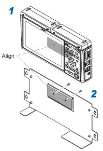
Secure the LR8450 (-01) by tightening the supplied screws (M3×5 mm) from the back of the stand.
