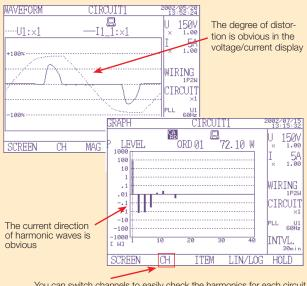
You can switch channels to easily check the harmonics for each circuit
