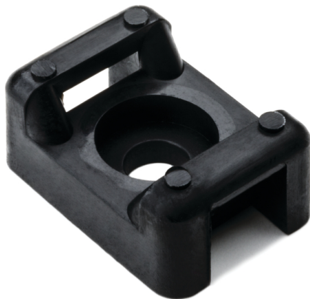
Cable Tie Anchor Mount, 0.86" x .61", 0.2" Hole Dia, 0.31" Max Tie Width, PA66, Black, 100/pkg
