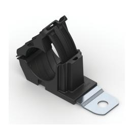
Ratchet P-Clamp, 0.76 - 1.42" Bundle Dia, 180° Short, 0.26" Hole Dia, PA66HIRHSUV/ST/ZN, Black, 3/bag
