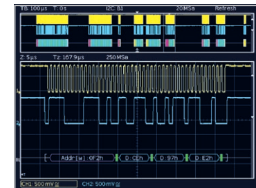
I 2 C bus hex decoding on the analog channel
