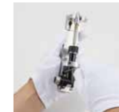
Perform positioning beforehand using the included jig.
