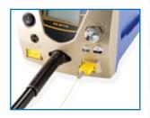
Two thermocouple inputs for integrated closed-loop process control.
