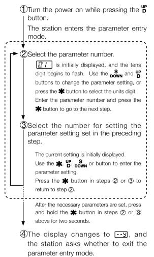
Select -3 and press the **\*** button to exit the parameter entry mode.
