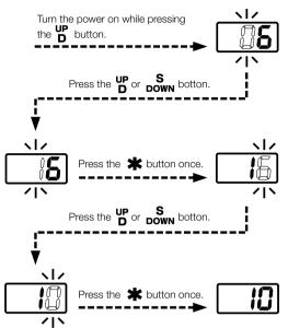
The channel D setting is completed as shown in the preceding diagram. Repeatedly pressing the the button moves to the channel S setting. (The process is the same as that for channel D.)
