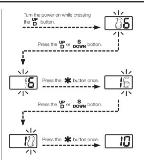
The channel D setting is completed as shown in the preceding diagram. Repeatedly pressing the \*\* button moves to the channel S setting. (The process is the same as that for channel D.)
