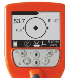
you will have the exact location of the transmitter and the lay of the pipe.
