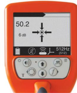
Simply follow the arrows to find the exact spot. When you are over the NULL point, the screen will produce this display.
