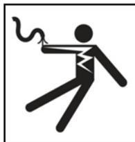
Electric shock resulting in death can occur if you plug this machine into an improperly wired outlet. If the ground wire is electrified, you can be electrocuted by just touching the machine, even when the power switch is off. A ground fault circuit interrupter will not protect you in this situation. Use a UL approved tester to determine if the outlet is safe.
