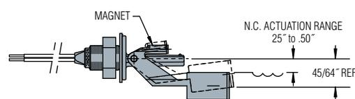
The LS-7 Type 12 is ideal for use on food warmers, hot water heaters, steam cookers, small boilers or wherever water evaporation occurs. The switch is used effectively for either high fluid level alarms or water make up systems.
