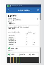
Switch port test shows switch name and IP address, connected port, and VLAN along with advertised speed and duplex settings. If a ping test is configured, the target address and average response time are shown. Scrolling down displays Power over Ethernet results.
