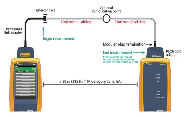
The patch cord adapters support Category 5e, 6, and 6A performance levels and work with all DSX CableAnalyzer™ models. The latest version of the Versiv/DSX firmware is required to use the MPTL testing limits.
