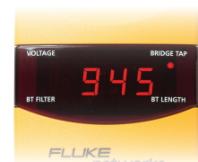
Bridge tap found at 945 feet /288 metres
