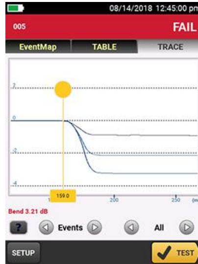
Bend as seen on an OTDR trace
