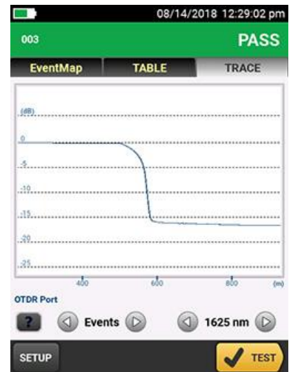
Splitter as seen on an OTDR trace
